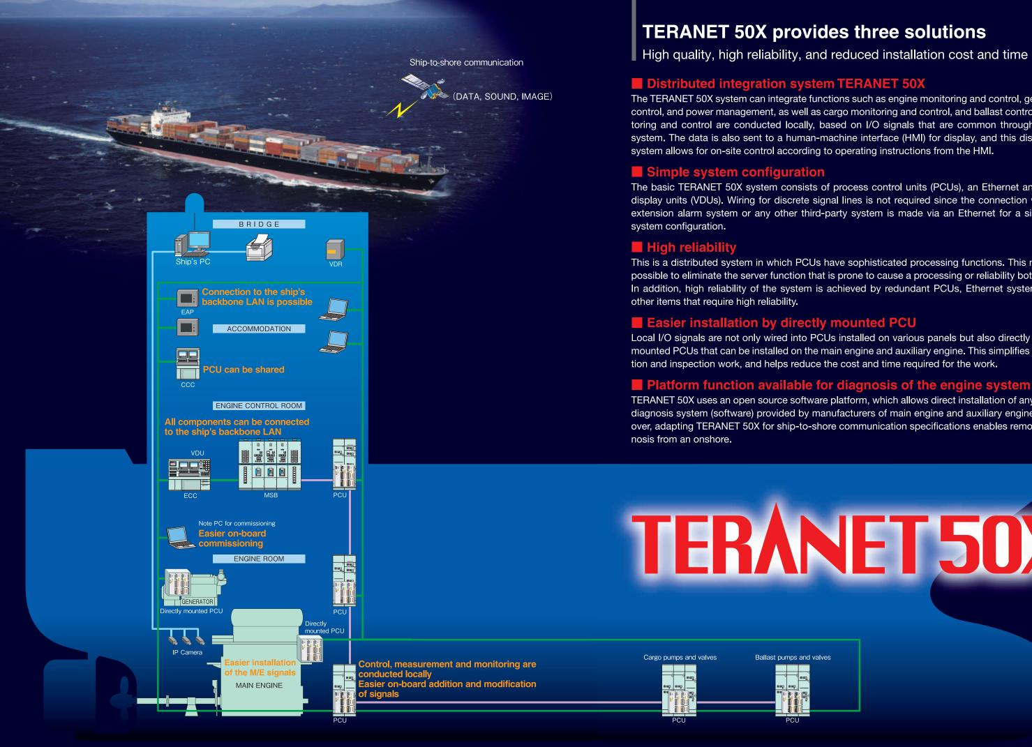
The TERANET 50X system can integrate functions such as engine monitoring and control, generator control, and power management, as well as cargo monitoring and control, and ballast control. Monitoring and control are conducted locally, based on I/O signals that are common throughout the system. The data is also sent to a human-machine interface (HMI) for display, and this distributed
